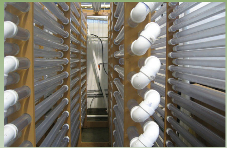
(clockwise from left) The machinery used for the ultra filter phase, phase 2, of the process after the manure leaves the digester and the bedding is created./ The final phase, phase 4, consists of reverse osmosis, which treats the water and gets it ready to discharge or incorporate into other by-products. / The bio-algae reactor that will be used to grow algae on the dairy.
