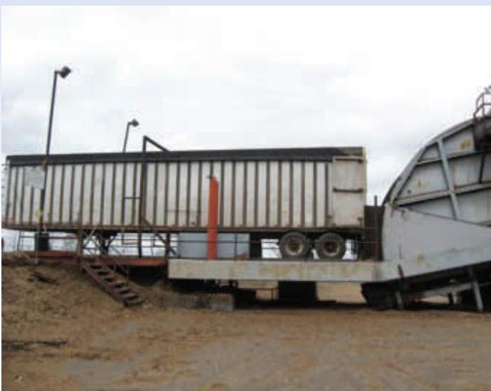
(left to right) Semi trailer parked on a lifting machine. / The hydraulic machine lifts the trailer in the air and the wood is dumped into a holding area. The process takes less than 15 minutes.
