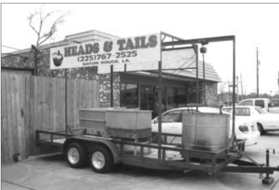
Figure 7. Custom mobile crawfish-boiling rig used for catering large crawfish boils.
