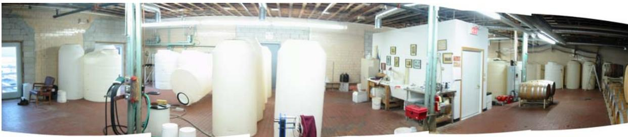
*South half of the cellar. Grape juice is pumped from the crush area into plastic barrels for fermentation. Barrel size is about 3 feet diameter by 6 feet tall holding about 320 gallons each.*
